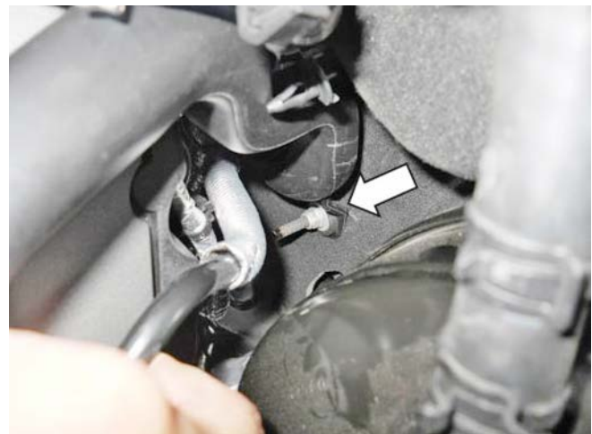
11. Using a 10 mm wrench or deep-well socket, remove the nut retaining the induction resonance tube to the firewall behind the driver side cylinder head.
