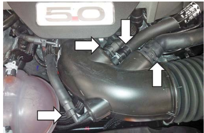
11. Using a 10 mm wrench or deep-well socket, remove the nut retaining the induction resonance tube to the firewall behind the driver side cylinder head.
