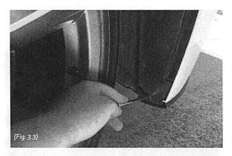
After removing the retaining pins, spread the fender liner to gain access to the bumper and install a J-clip (Nipple side is toward the front of the car) at each of the three holes in the bumper.
