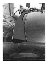
Step 5: Install rear spoiler by centering spoiler around rear brake lamp. Spoiler is slightly smaller than width of glass. Do not remove red backing from tape until fitment is confirmed.
