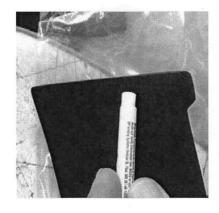
Step 2: Apply the provided 3M adhesive promoter onto the part and press the tape on.
