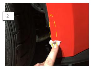
Clean the tape mounting surface with the supplied alcohol wipe. Allow time for the surface to dry. Then apply the supplied adhesion promoter and allow it to haze.
