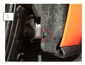
Raise and support the rear of the vehicle. Remove the factory splash shield retaining clip.
