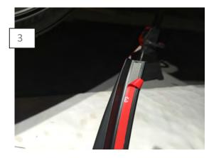
Peel off the tape backing. Position the Splash Shield and secure with the supplied push pin. Apply firm even pressure on the double sided tape to ensure proper adhesion.
