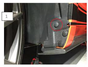
Raise and support the front of the vehicle. Turn wheel for better accessibility to the mounting locations. Begin by removing the factory push pin circled above.
