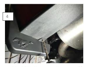
From below, drill the addition mounting location using a 1/4" drill bit. Mount using the supplied push clip.
