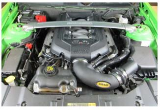
**11.** Reinstall the engine cover and Reinstall the strut tower brace, if so equipped. Reconnect the Battery terminal.
