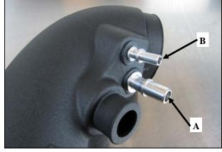
**5.** Install the Grommets and Fittings into the Modular Intake Tube. **A)** All models will require the use of the 5/8" Fitting and the 5/8"Grommet. **B)** Automatic transmission equipped vehicles will also use the 3/8" Fitting and 3/8" Grommet.
