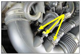
**3.** Compress the spring clamp and disconnect the resonator from the air intake tube. Carefully depress the connector lock tabs, and disconnect the crank case breather line and the brake aspirator line if equipped, (AT models only).
