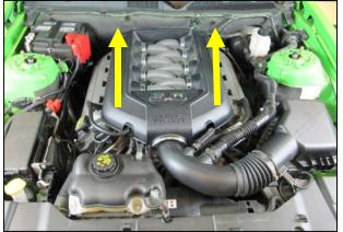
**2.** Lift straight up on the engine cover to unseat it from the mounting grommets and set it aside.
