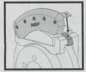
Place the cover over the caliper and position hole in bridge over the threaded stud and onto the clip (may require minor flexing to pull second hole over stud).
