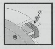
Install the supplied locknuts onto the threaded studs to secure clip to bridge. Tighten with 3/8-inch wrench or socket to 25 inch pounds. Over tightening could pull stud through aluminum bridge.
