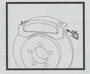
Slide the stainless steel clips on each side of the brake caliper bracket. Fit should be snug and secure.
