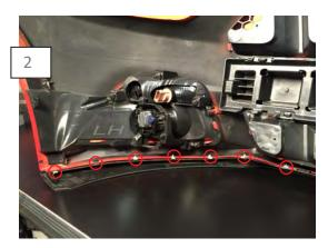
Remove the fasteners holding the chin spoiler to the bumper. Base and Performance pack cars are secured using similar hardware.
