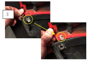
Transfer the screw clip from the factory chin spoiler to bumper cover as seen above.
