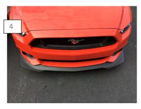
Install the GT350 Style Chin Spoiler using the factory hardware, then reinstall the factory splash shield.
