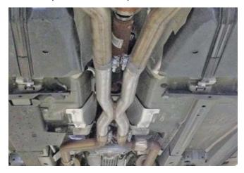
Before starting the vehicle, make sure to check all wires, hoses, brake lines, body parts, tires, and any other components for safe clearance from the exhaust system.
