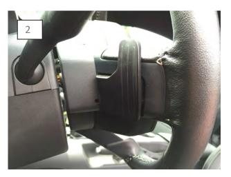
Clean the mounting surfaces with the supplied alcohol, allow time to flash dry.
