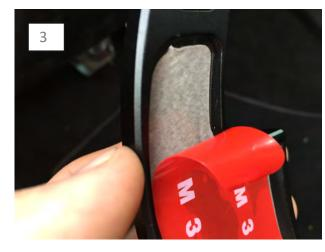
Peel back the adhesive backing. Line the extension up with the factory paddle shifter.
