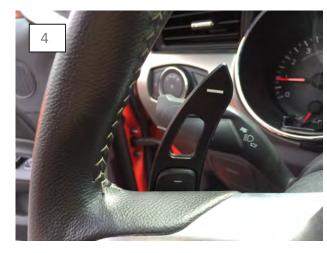
Apply firm pressure to the paddle and paddle extension to ensure proper adhesion.
