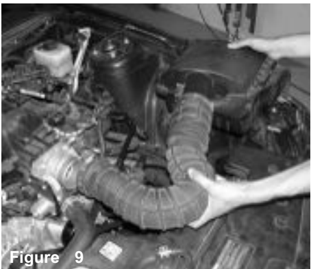
Figure 6 The crank case hard pipe breather line is disconnected.
