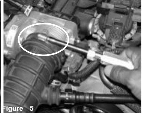
Figure 5 The clamp on the air intake duct is loosened.
