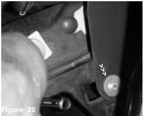
Figure 17 The heat shield bracket is secured with the stock bolt removed earlier.
