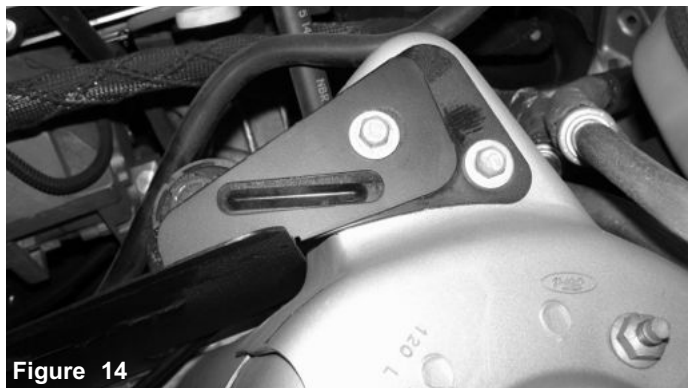
Figure 12 The heat shield is now lowered into the engine compartment and brackets are aligned.
