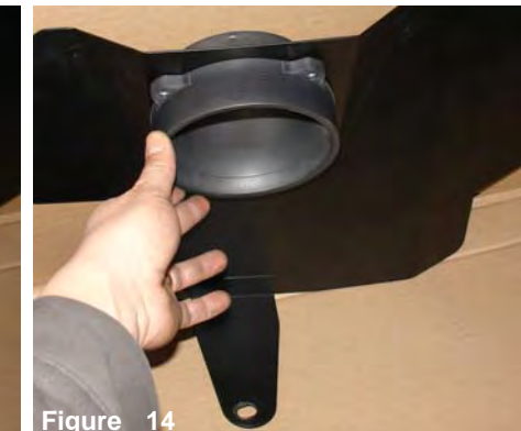
Figure 14 The velocity stack m6 inserts are aligned and the velocity stack is sitting flush with the heat shield.
