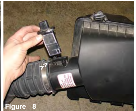
Figure 8 Carefully, remove the mass air flow sensor from the sensor housing.
