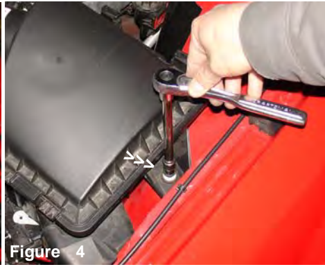
Figure 4 Loosen and remove m6 bolt holding the air box cleaner to the fender well.
