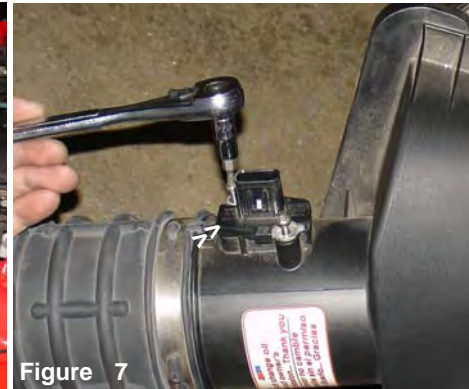
Figure 7 Use the T20 torx bit in this kit to remove the two screws holding the mass air flow sensor in place.
