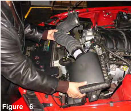
Figure 6 Once the clamp and bolt have been removed, continue to remove the entire air box assembly from the engine compartment.
