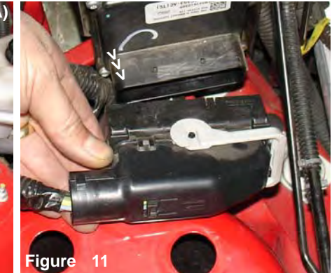
Figure 11 Unlatch the white brace holding harness to the ABS solenoid. Set the harness to one side until the heat shield has been installed.
