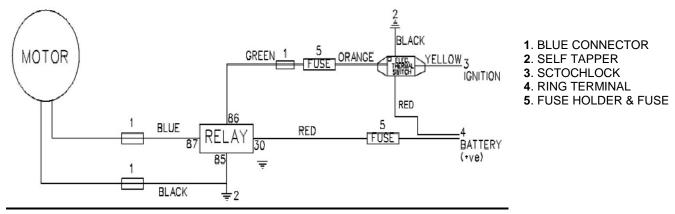
WARNING: ENSURE IGNITION SOURCE IS NOT CONNECTED TO THE ENGINE MANAGEMENT SYSTEM
