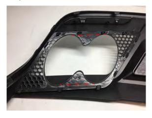
**Step 21:** Install the bumper in reverse order. Ensure this connector doesn't get pinched between the bumper cover brace and the metal bumper otherwise, the bumper will not fit correctly.
