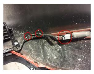
Step 11: Unclip the license plate light housing and trunk button.
