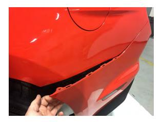
**Step 8:** Firmly pull the bumper from the vehicle. The top edge of the bumper is only held on by clip pressure.
