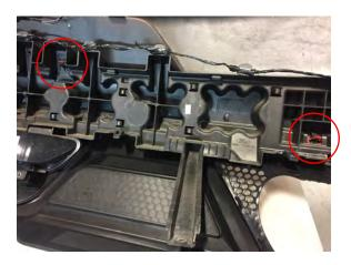
**Step 13:** Transfer the screw clips from the factory bumper over to the diffuser.
