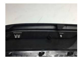
**Step 19:** Clip the bumper brace with the wiring harness to the new bumper. It will clip on using the factory center clip locations.
