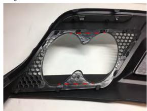
**Step 12:** Reinstall the diffuser to the bumper in the reverse order.
