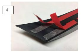
Remove the tape backing from the insert, install the insert onto the vent.
