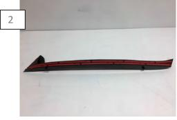
Prepare the fender vent by first installing the Fender Vent insert. Test fit the insert on the vent. Remove the insert and apply the supplied 3M double sided tape.
