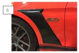
Peel off the double sided tape backing and apply the vent to the vehicle. Apply firm even pressure to ensure proper adhesion.
