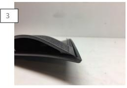
Test fit the insert again, ensure sure the end sit flush with the vent otherwise, the vent will not fit correctly on the car.
