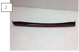
Apply the supplied 3M tape to the scoop insert. Test fit the insert on the scoop to familiarize yourself with how it fits. The insert edges need to be flush with the scoop otherwise, the scoop will not fit correctly.
