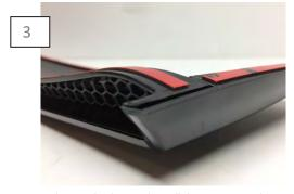
Remove the tape backing and install the insert onto the scoop.
