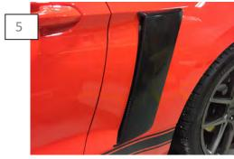
Test fit the scoop before removing the tape backing. Once your comfortable with how the scoop fits, remove the tape backing. Apply firm even pressure to ensure proper adhesion.
