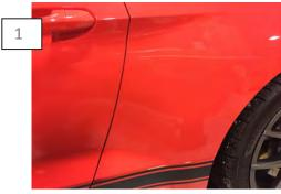
Wash the rear quarter panels with soap and water. Allow the panel and surrounding area to dry. \*\*Recommended: Wipe the panel down with isopropyl alcohol to ensure the cleanest surface possible.
