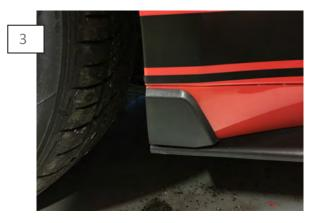
Remove the 3M tape backing, install the winglet onto the fender. Apply firm even pressure to ensure proper adhesion.
