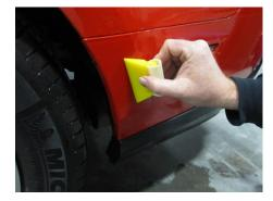
This completes the installation of your 3M Paint Protection Film. Do not wash the vehicle for 24 hours prior to application. Never use pigmented or paste waxes on the film.
