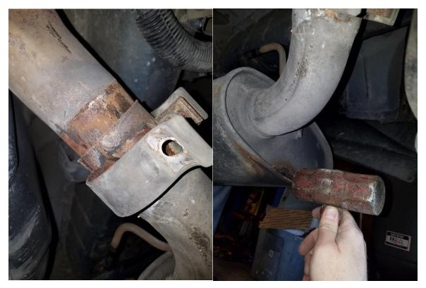
• Remove the factory muffler from the rubber hangers pulling towards the front of the car.
