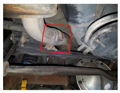
Next locate and loosen the clamps on the factory mid pipe towards the catalytic converters, using 15mm socket and ratchet. Do not remove, this is just temporary while installing and adjusting new mufflers. Again, penetrating oil will help slide the clamps towards the rear of the car with a hammer and screwdriver for clips on clamps.
