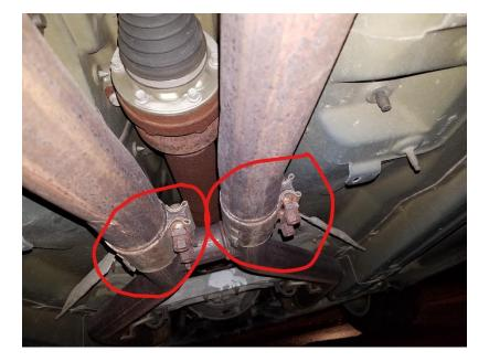
• Using a hammer and a chisel or a pry bar, remove the factory mufflers from the mid pipe. (Having the mid pipe loose and hanging from the front exhaust system helps a lot with removing the mufflers. Two people, one to pull each way on the pipe and muffler, while twisting.)
