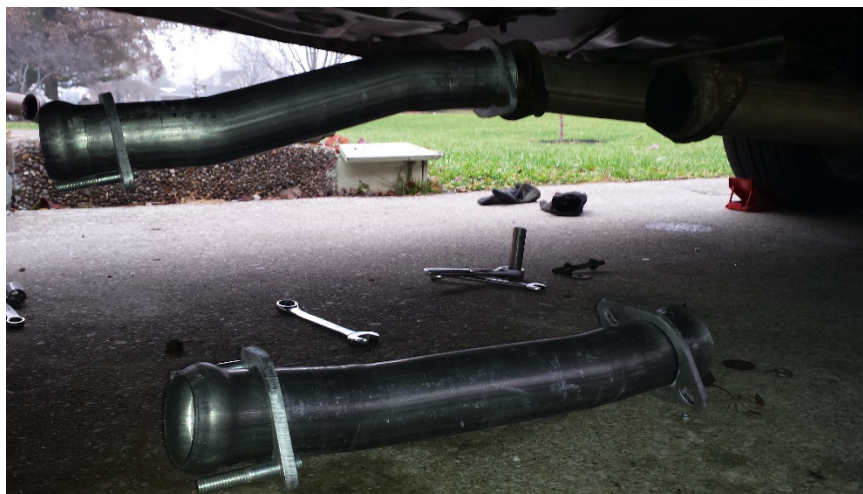
7. Mount flow tubes to mid-pipe using old bolts, or purchase ones if needed.
