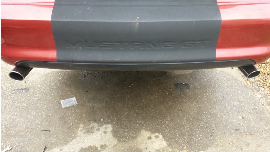
MAC 3" tips were long enough to have about 1.5" protruding from rear bumper on a 1995 GT.
