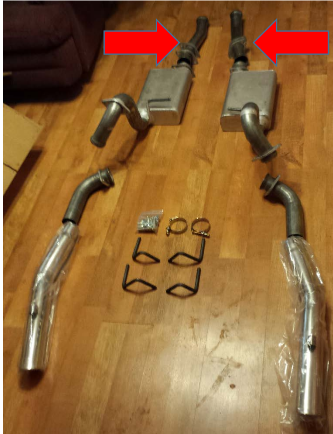
7. The two flow tubes are identical.
