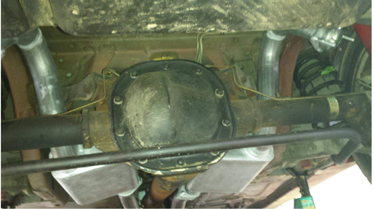
9. Underside view of mufflers properly mounted to rubber hangers and flow tubes.
