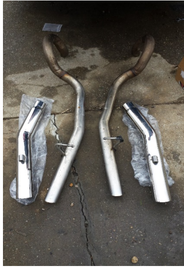
Side by side comparison of factory 2.25" tips with MAC's 3" tips.
