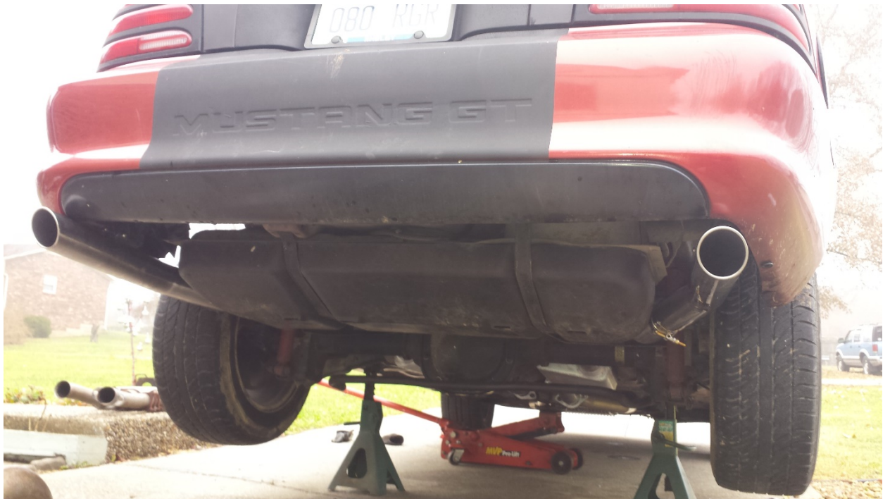
Completed shot of MAC Catback with 3" exhaust tips on a 1995 GT.
