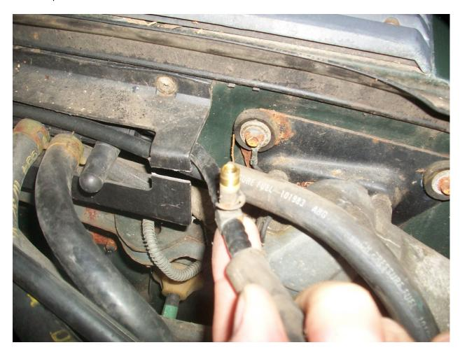
2. Locate the stock fuel pressure regulator. This will most likely be attached to the fuel rail. It will have small black vacuum line coming from the top. In this picture it is the brass colored item on the left near the intake runners.
