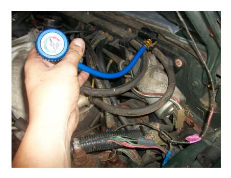
9. Start the vehicle. Using a 1/8 Allen wrench, adjust the fuel pressure to the factory setting of 43 PSI. Modified cars will require extra fuel pressure and stock cars usually respond better to slightly lower pressure. Fuel pressure in excess of 60 PSI is not recommended for street applications.
