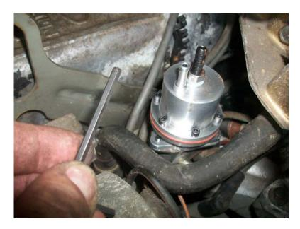
10. When the desired setting is reached you can hand tighten the silver lock nut on the adjustment screw to keep your setting. Reattach the vacuum line and use your pliers to secure the retaining clip. The fuel pressure should drop approximately 1 PSI for each PSI of vacuum.
