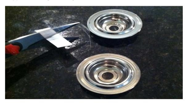
(4) Apply Butle Tape based on Trial Fit where contact with Strut Tower occurs.
