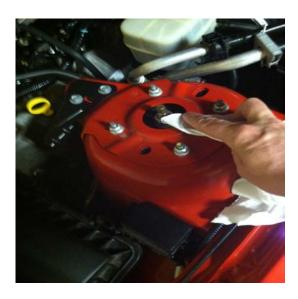
(2) Insure Strut Covers are clean prior to applying Butle Tape. (Note: Trial fit Strut Covers to insure proper fit prior to applying Butle Tape)
