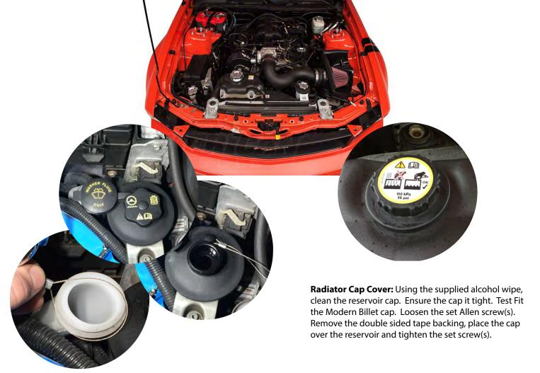
**Windshield Reservoir / Power Steering Cap:** Remove the factory reservoir cap. Wrap the cable tether around the reservoir opening then press the cap onto the reservoir.
