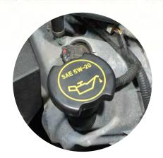
**Oil Cap Installation**: Remove the factory oil cap by turning it counter-clockwise. Then Install the Modern Billet Chrome Oil Cap.
