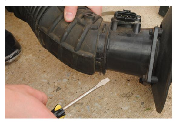
16. Remove the (4) bolts around the base of the sensor and you will have the part you need.
