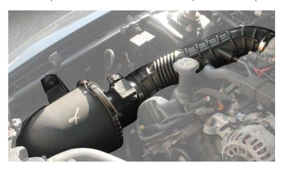
8. Remove the entire intake housing from the vehicle. This may require some wiggling and twisting, but it shouldn't be too hard to remove from the car.
