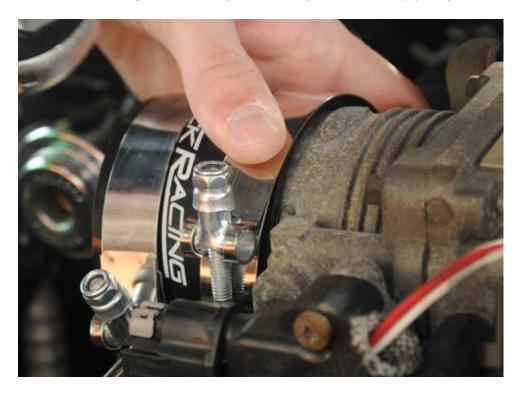
12. Before you install the new 3" Stack Racing intake into the vehicle, remove the intake air temperature sensor from the old housing. Install the sensor in the rubber mount on the new 3" intake pipe.
