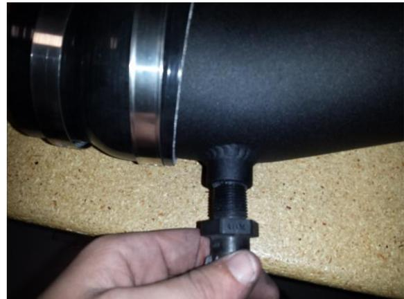
Step 4. Screw the factory IAT sensor into the new upper intake tube
