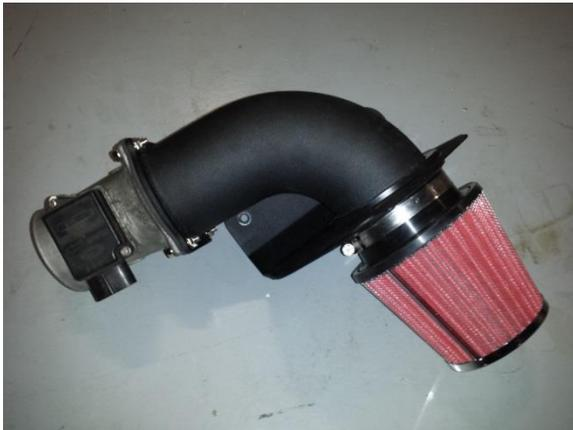
Step 2. Install the MAF sensor onto the lower portion of the intake tube then install the heat shield and filter onto the tube.
