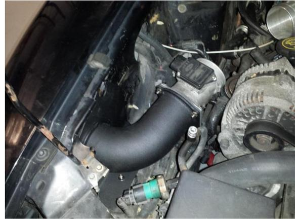
Step 3. Place the lower portion of the intake into the fender well and secure it to the vehicle using the factory mounting points.
