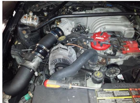
Step 5. Install the upper portion of the intake onto the vehicle, ensuring all connections are plugged in and tight before driving the vehicle.
