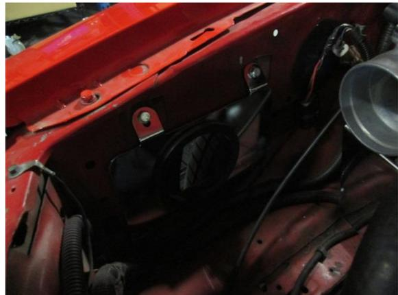
Step 4. Install the heat shield onto the fender wall and secure it using factory hardware.
