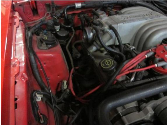
Step 1. Remove your factory intake and MAF sensor from your vehicle. The MAF sensor housing will need to be reused in the new intake assembly.
