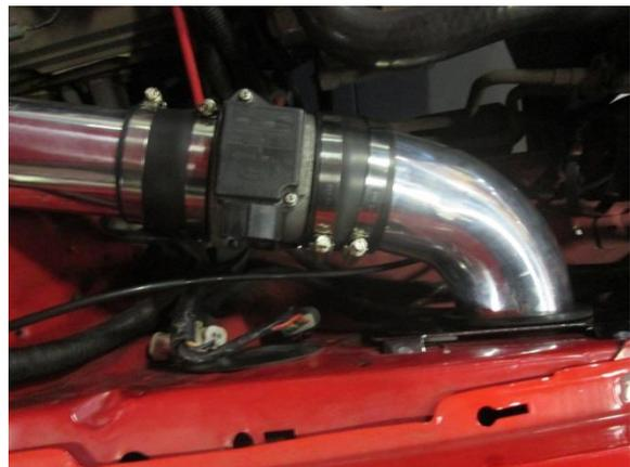
Step 5. Slide the lower intake tube onto the MAF and then position it into the heat shield. Once it is secure, install the filter onto the tube and tighten all couplers down.
