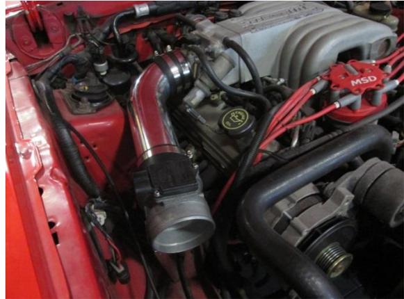
Step 3. Install the MAF onto the intake tubing using factory mounting hardware.
