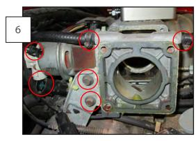
Remove the EGR electrical connection, EGR vacuum line, (2) regular screwdriver hose clamps with coolant hoses and (2) 10mm throttle cable bracket bolts. (Coolant may still be in the hoses.)
