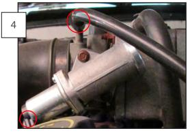
Unplug the rubber breather hose from the top of the throttle body. Unplug the electrical connector on the bottom of the idle air control valve.
