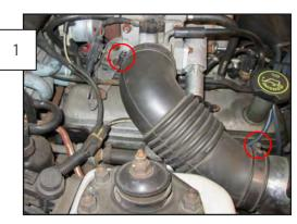
Remove the (2) regular screw head, hose clamps on the stock, black air hose. Remove the upper air hose from the vehicle.
