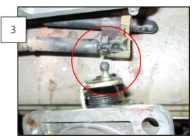
Remove the throttle cable by pulling it away from the throttle body.
