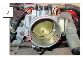
Remove the (4) 1/2" nuts from the throttle body.
