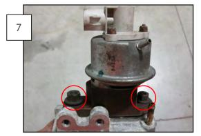
Remove the (2) 9/16" EGR nuts from the Exhaust Gas Recirculator. Clean off the old gasket material from the EGR and place the EGR on the new spacer with a new gasket. Tighten the nuts on the new spacer using a 13mm and a 17mm socket.
