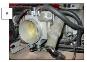
Reinstall all of the components on the new EGR spacer. Use the included throttle body gasket and spacer/instake manifold gasket to install it back on the intake manifold. Reinstall the components to the throttle body and install it to the EGR spacer. Reinstall the upper air hose and plug in all electrical connectors. Reconnect the negative battery cable. Re-adjust the Engine Idle Speed.
