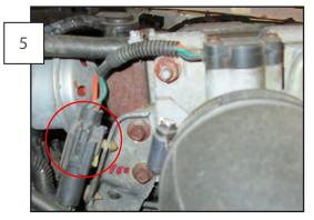
Remove the THROTTLE POSITION SENSOR by unplugging the electrical connector . Place a rag under the throttle body to soak up coolant and carefully remove it from the vehicle.
