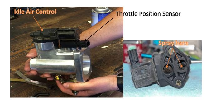
8. Install throttle position sensor and idle air control (with supplied gasket) onto new throttle body. Note: After all installed, if your car idles to high or too low, it is very likely that your throttle position sensor isn't adjusted right.
