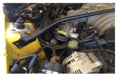
3. Detach the 3 cables/linkages to the throttle linkage
