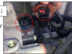
Unplug the Idle Air Control and Throttle Position Sensor electrical connectors.
