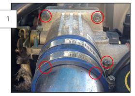
Remove the (1) upper intake tube hose clamp. Move the tube out of the way from the throttle body. Remove the (4) 13mm throttle body reaining nuts.
