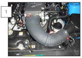
Disconnect battery before beginning installation. Remove factory air intake assembly.
