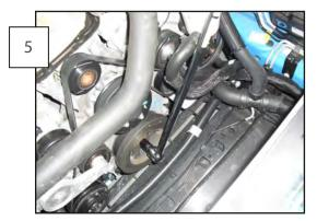
Using an 18mm socket and a breaker bar (or an impact gun), loosen the crankshaft bolt.
