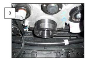
Make sure crankshaft snout is clean before installing new balancer. Apply a light bead of high-temp RTV silicone to keyway on Stack Racing balancer, then slide balancer onto crankshaft snout. The balancer will not be fully seated at this point, follow instructions in Step 9 closely to pull the balancer fully onto crankshaft snout.
