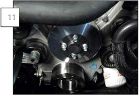
Install the new water pump pulley using the factory bolts, making sure to check clearance of the stud that was trimmed in Step 10.
