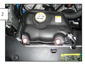
Remove factory coolant overflow bottle by removing the 8mm bolt and 10mm bolts holding it to the fan shroud.
