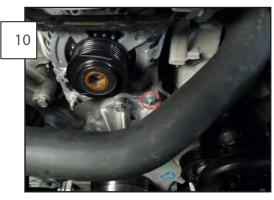
In order to make clearance for the new water pump pulley, you must grind down one of the water pump studs for clearance. You can either use a Dremel or Rotary Tool to cut the stud on the car, or you can remove and use a hacksaw. Shown below is the stud before and after trimming.
