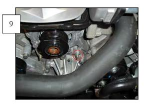
Using the supplied bolt and factory washer, tighten until the factory bolt can be safely threaded into the crankshaft snout. Do not over-tighten supplied bolt, it is only to be used to draw the balancer far enough onto the snout until the factory bolt and washer can safely be threaded into the snout. Once balancer is fully seated, use the following procedure to properly torque the bolt to Ford factory specs:
