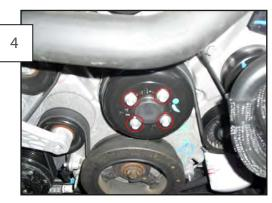
Loosen the four water pump pulley bolts using a ratchet and 10mm socket.
