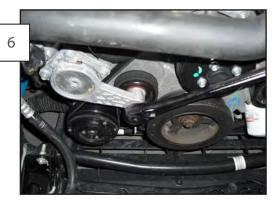
Once the crank bolt has been loosened, use a 1/2" drive ratchet to remove the accessory drive belt.ch.
