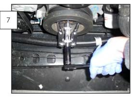
Once the belt has been removed, fully remove the factory crank bolt and washer. Re-thread the bolt without the washer about halfway into the crankshaft. Use a three prong pulley puller tool to remove factory balancer from crankshaft.
