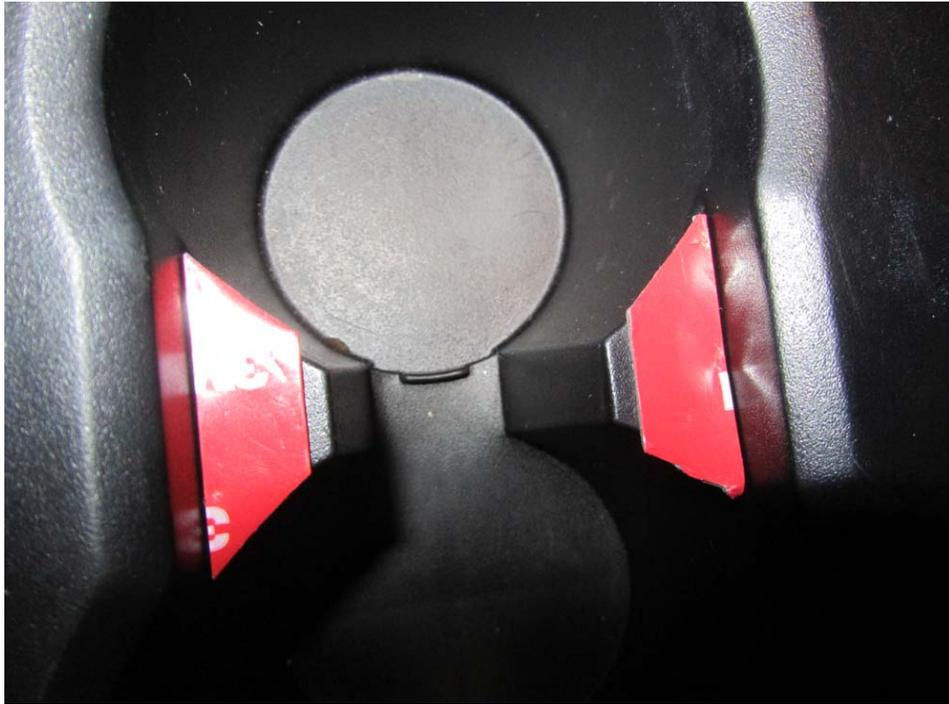
3. Press down on tape firmly when satisfied with alignment. Peel away the top red wrapper on the double-sided tape.
