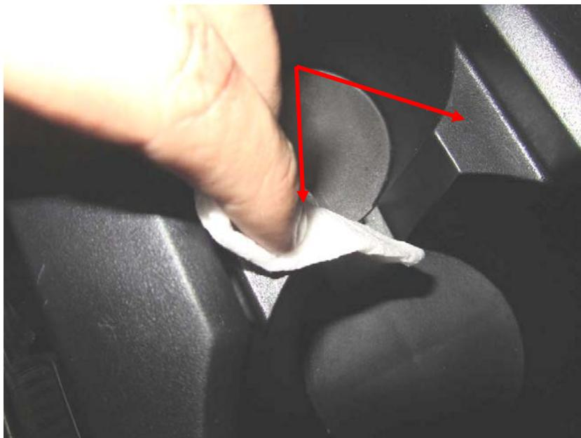
2. Line up the double-sided tape on top of the plastic that is on the inside of the cup holders. Next, cut out the double-sided tape along the lines of the plastic so that when the bezel is placed inside the cup holder, there is no tape showing below it.
