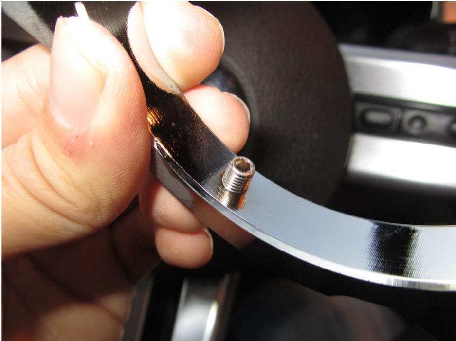
5. Wipe off the bottom right and left hand side of the bezel where the bottom will come in contact with the double-sided tape.
