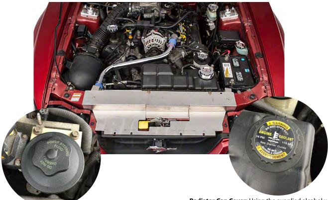
**Power Steering Reservoir Cap:** Remove the factory reservoir. Wrap the cable tether around the reservoir opening then press the cap onto the reservoir.
