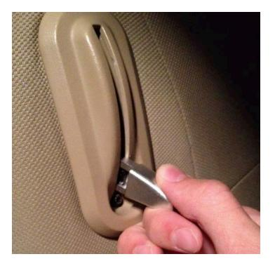
**NOTE:** After installing your new aluminum seat release levers, they may stick slightly in the track when pulled upward because of the wider contact area. The sharper metal edges may scrape off small amounts of plastic, but this is not noticeable and once they have been worn in, will function equally to the old levers and look great. If you prefer, you can run the new levers up and down the track to wear them in immediately after installation.
