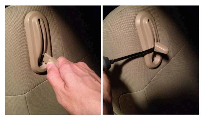
**Step 3:** To attach the new levers, have the less rounded side facing upward and simply push the new levers onto the small metal piece inside the track. They will stay snugly attached.
