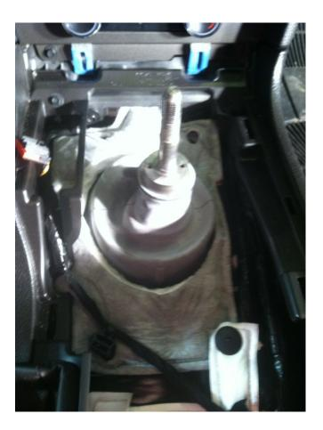
5. Remove the plastic connectors that attaches to the sound insulation.
