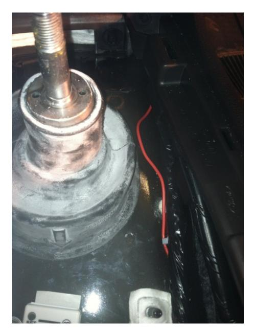
9. Run the positive (red) wire along the right side of the gear shift and behind the plastic panel.
