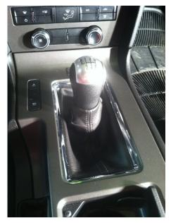
1. Begin by taking off the factory shift knob by unscrewing it counter clockwise.
