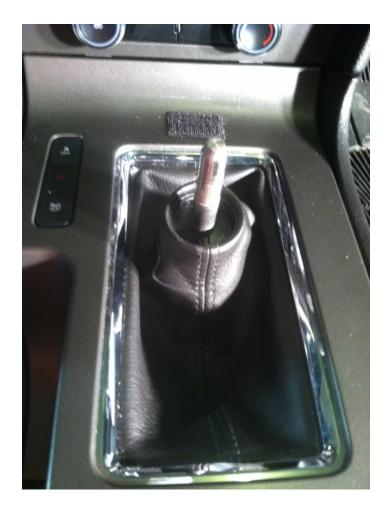
2. Once off, open up the arm rest and pull up on the plastic to pop the center console off.
