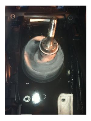
7. Take the 10mm socket and socket wrench and partially remove the bolt to the bottom left of the gear shift.
