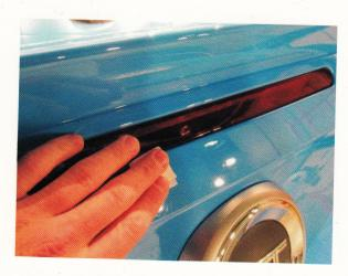
**Step 2:** Peel the backing from the 3M tape and place the trim over the 3<sup>rd</sup> brake light. Once properly positioned, press down firmly to fully seat the adhesive tape.
