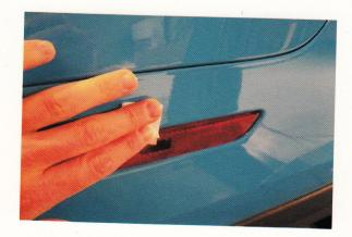
**Step 2:** Peel the backing from the 3M tape and place the trim over the quarter light. Once positioned properly, press down firmly to fully seat the adhesive tape.
