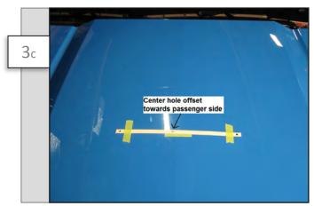
Once in the correct position, tape the template to the hood as shown. (*Make sure center hole is offset towards passenger side as seen above*)
