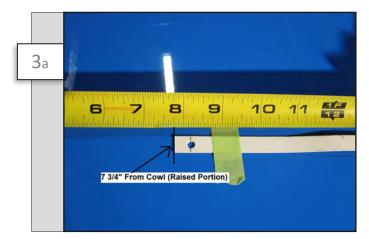
Measure 7 %" from the edge of the cowl (raised portion of hood) on either side to center the drill template.
