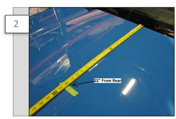
Use a tape measure and masking tape to mark a spot 22" in the center of the hood from the rear.
