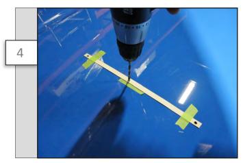
Using a 3/16" bit, drill 3 holes through the hood using the template as a guide. Use a shop-vac to clean up any metal shavings after drilling.
