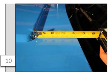
Remove the backing from the adhesive strips and place the scoop on the hood using the pre-drilled holes as a guide. (DONT PRESS DOWN YET)
