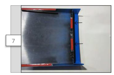
Remove the backing from the adhesive on the scoop's insert and install it on the front of the scoop as shown. Place the final two adhesive strips to the underside of the insert.
