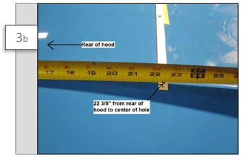
Measure 22 3/8" from the rear of the hood to the center of the hole on the template to align it.
