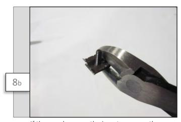
If they are loose on the insert, squeeze the backside with a pair of side cutters to tighten the gap.
