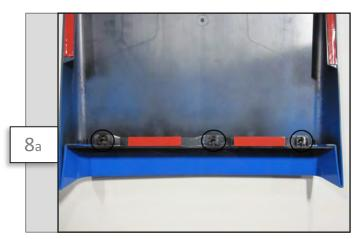
Install the 3 included U-Studs on the scoop insert.
