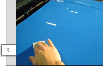
Thoroughly wipe the area of the hood where the scoop will be applied with the supplied alcohol pads to ensure a clean bond.
