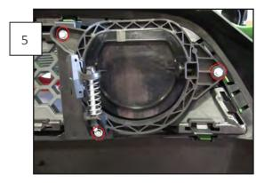
Re-install the bracket onto the grille assembly using the three 7mm screws removed in Step 1. Be sure that the delete plate is flush with the factory fog light opening before fully tightening the screws.
