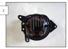
Remove the five T15 Torx Head screws securing the LED resistor housing to the fog light and carefully remove it.
