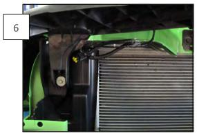
Repeat Steps 1-5 for the opposite side fog light delete. Find a safe place in the upper radiator support to secure the factory fog light harnesses so they cannot be seen and are protected from the elements.
