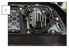
Remove the three 7mm screws securing the fog light bracket to the grille assembly and remove it from the grille with the fog light still attached.
