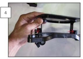
Install the delete plate in the bracket by placing one side over the post in the bracket and snapping the other side in as shown.
