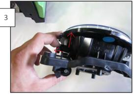
Pull back the tab on the fog light bracket to release the light as shown.
