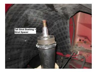
**Option 2:** This raises the strut mounting point from a stock setting. Use with cars at stock height to cars slightly lowered (.5" - .75").
