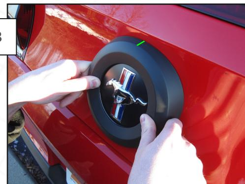
Install the cover over the emblem as shown, making sure the thicker wall (marked by a green line) of the cover is at the top. Once the cover is properly aligned, press down firmly around the edges to fully seat the tape.
