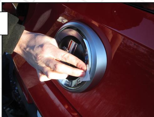
Using the supplied alcohol prep pad, thoroughly wipe down the chrome plated area of the emblem where the cover will adhere.
