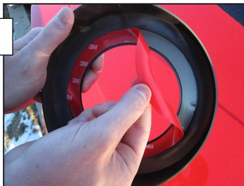
Remove the tape backing by pulling on the small tab as shown.
