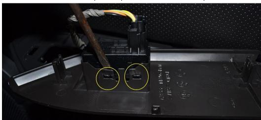
\*\*Note: The plastic clips is thin so it can break easy\*\*
