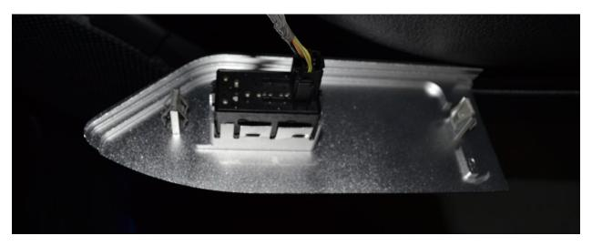
\*\*Note: You may need to bend the clips back on the new plate to allow the module to be installed, then you can bend the clips back in to secure the module in place\*\*
