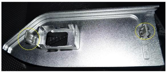
The clips will be tight to put on, you can use the handle side of the screw driver and tap the retainer clips on the new switch to keep them secure.
