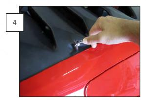
Once the louvers are in the proper position, firmly press down to fully seat the adhesive tape on the brackets. Using an 8mm socket and ¼" drive, tighten the nuts to secure the louvers to the brackets. Do not over tighten the nuts, just past snug is enough. Cleaning: To clean your rear window, simply remove the 8mm nuts/washers and remove the louver from the vehicle.
