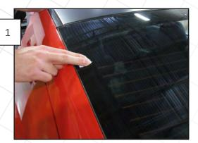
Wipe down the outer edge of the rear window with the supplied alcohol prep pads where the louver brackets will adhere. Once dry, follow with the supplied 3M Adhesion Promoter.
