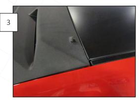
Open the trunk before installing louvers. Pull the backing from the 3M tape on the brackets and place the louvers over the rear window (Do not let the tape adhere to the window yet). Line up the corners of the louver with the upper corner of the rear window as shown.
