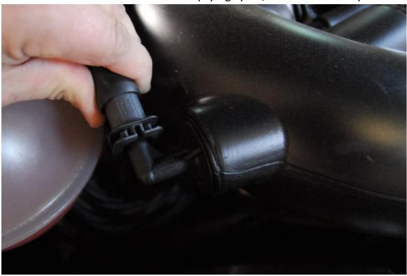
3. Loosen the screen on the air intake and separate from the throttle body. You can move it out of the way enough to work, so no need to completely remove it.
