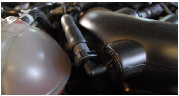
To do this, simply rotate the clip until you can see the bottom clips. Insert a flathead screw driver into both sides prying apart, then work the clip out.
