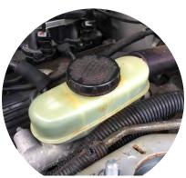
**Brake Fluid Reservoir Cap:** Using the supplied alcohol wipe, clean the reservoir cap. Ensure the cap it tight. Test Fit the Modern Billet cap. Loosen the set Allen screw(s). Remove the double sided tape backing, place the cap over the reservoir and tighten the set screw(s).
