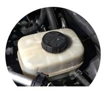
**Brake Fluid Reservoir Cap:** Using the supplied alcohol wipe, clean the reservoir cap. Ensure the cap it tight. Test Fit the Modern Billet cap. Loosen the set Allen screw(s). Remove the double sided tape backing, place the cap over the reservoir and tighten the set screw(s).
