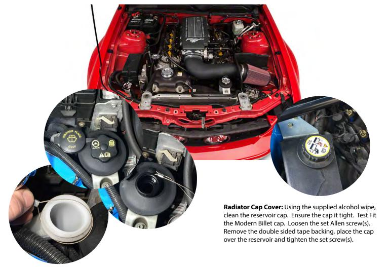
**Windshield Reservoir / Power Steering Cap:** Remove the factory reservoir cap. Wrap the cable tether around the reservoir opening then press the cap onto the reservoir.
