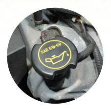
**Oil Cap Installation**: Remove the factory oil cap by turning it counter-clockwise. Then Install the Modern Billet Chrome Oil Cap.
