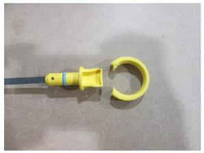
**STEP 2.** Using a small hand saw, cut the top of the handle off where you previously marked it and trim the sides to be square in shape.
