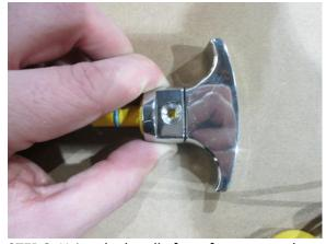
**STEP 3.** Using the handle for reference, mark the factory handle for drilling.
