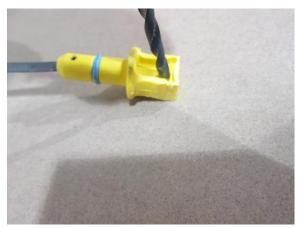
**STEP 4.** Using a 5/32 drill bit, drill a hole for the retaining screw to pass through.
