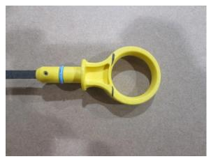
**STEP 1.** Measure from the base of the dipstick handle up 5/8" and mark the handle for cutting.
