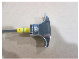
**STEP 5.** Slide the t-handle over the factory handle and insert the retaining screw into place to hold the two halves together.
