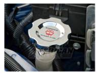
**Brake Fluid Reservoir Cap:** Using the supplied alcohol wipe, clean the reservoir cap. Ensure the cap it tight. Test Fit the Modern Billet cap. Loosen the set Allen screw(s). Remove the double sided tape backing, place the cap over the reservoir and tighten the set screw(s).
