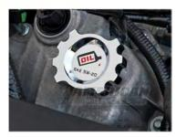
**Oil Cap Installation**: Remove the factory oil cap by turning it counter-clockwise. Then Install the Modern Billet Chrome Oil Cap.
