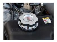
**Radiator Cap Cover:** Using the supplied alcohol wipe, clean the reservoir cap. Ensure the cap it tight. Test Fit the Modern Billet cap. Loosen the set Allen screw(s). Remove the double sided tape backing, place the cap over the reservoir and tighten the set screw(s).
