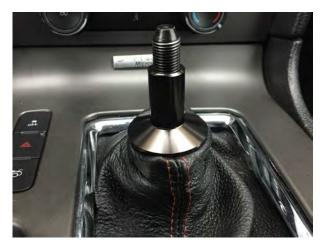
Install the supplied shift boot retainer. Thread the retainer on as far as it will go. Pull the shift boot onto the groove of the retainer.
