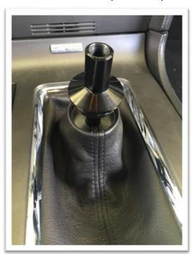
**4.** Insert the shift knob retainer turning it clockwise until it stops all the way down the shifter handle.
