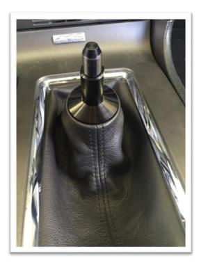
**5.** Install the shift knob turning it clockwise until it stops, DO NOT TIGHT IT, then return it turning it counterclockwise until a desired position is obtained.
